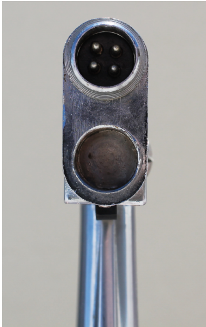
Illustration 2: The four-pin screw-on connector on the base.
