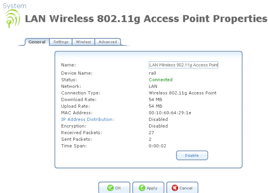
Figure 8.60. LAN Wireless 802.11g Access Point Properties -- Enabled
