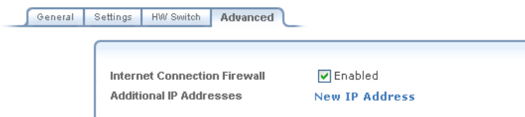
Figure 7.94. Apply Firewall Protection
