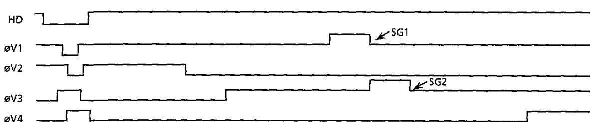
Figure 5-6. Charge Read-Out Timing Chart
