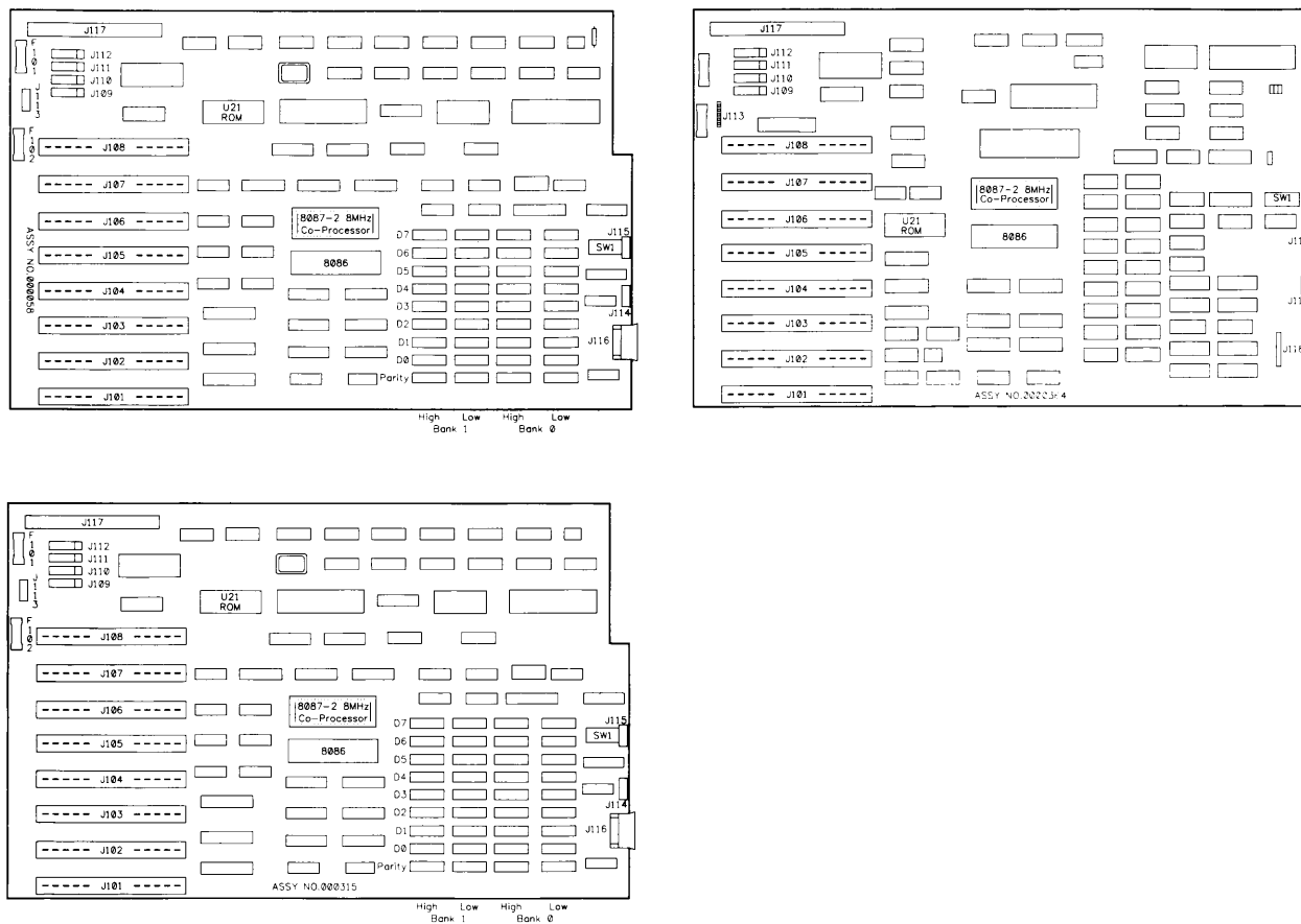
Figure 7-30. COMPAQ DESKPRO System Boards (assy. no. 000058, 000315, and 000364).
