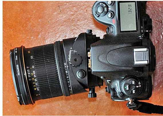
The PC-E Nikkor 24mm f/3.5D ED Lens of 2008 adds the tilt function to Nikkor's traditional shift function
