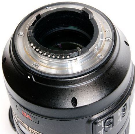
The flange of a current F-mount lens, including aperture lever (upper left) and CPU contacts (bottom).
