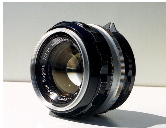
A typical F-type ("Pre-AI") lens, the Nikkor 50mm 1:1.4 showing "Nippon Kogaku Japan" engravings, scalloped-metal focus ring, and old-style Meter Coupling Prong (clearly visible to the top right of photo).
