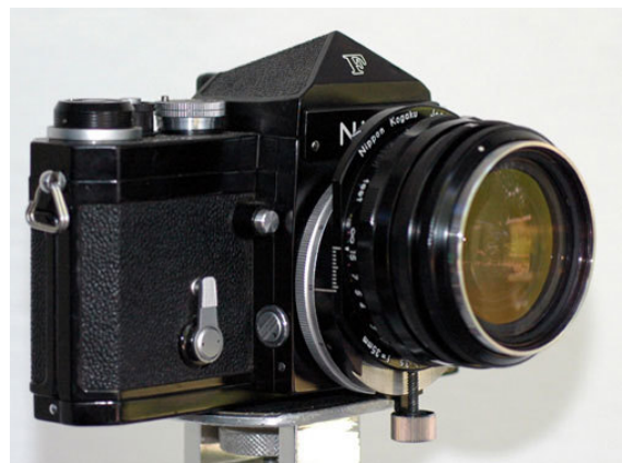
The 35mm f/3.5 PC-Nikkor, introduced in 1961. Note the small clearance between the shifting section of the lens and the camera body. The lens cannot be mounted on later camera bodies with protruding prisms.
